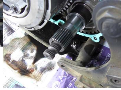
With the Clutch casing back on and tightened back up the O seal on the starter gear casing was damaged so we replaced it and then bolted it back on
