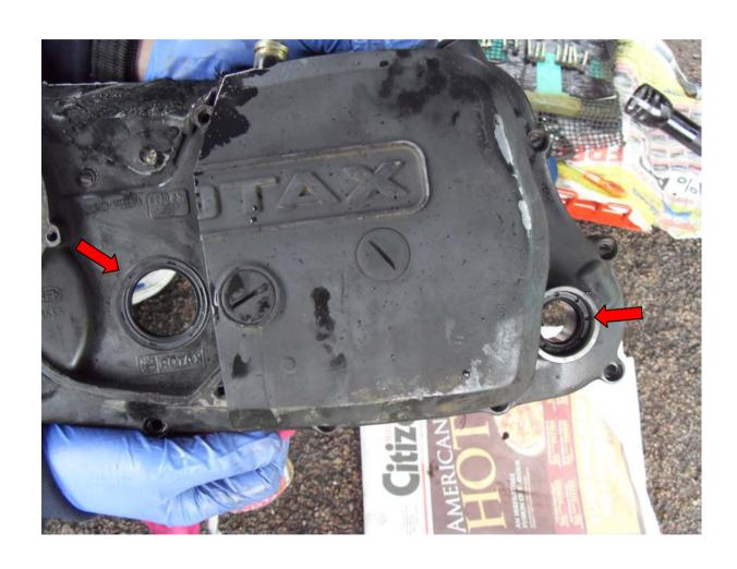
Now the reassembly started and the gasket is put in place and all the kick-start and gear shafts were cleaned up so not to get grit on the new oil seal.
