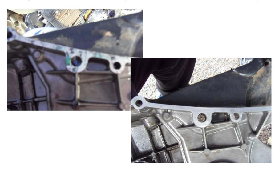
As the Clutch casing was of and the history of this bike is not to well known the oil seals were also changed the kick start oil seal (RIGHT) and the lower cam belt Pulley oil seal (LEFT)
