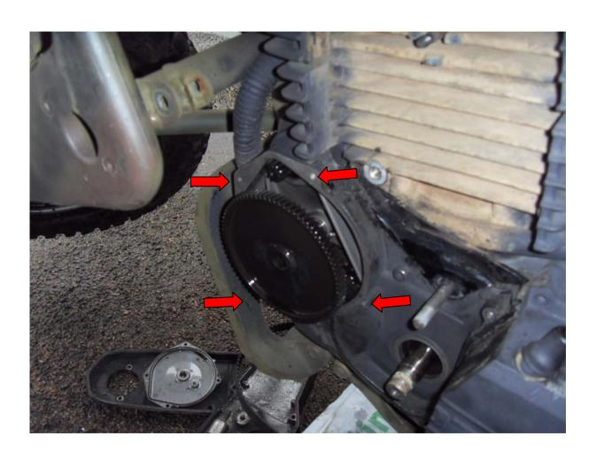
with all the Cap heads Removed the last thing to do is remove the Cir clip and O ring from the kick start and gear leaver
