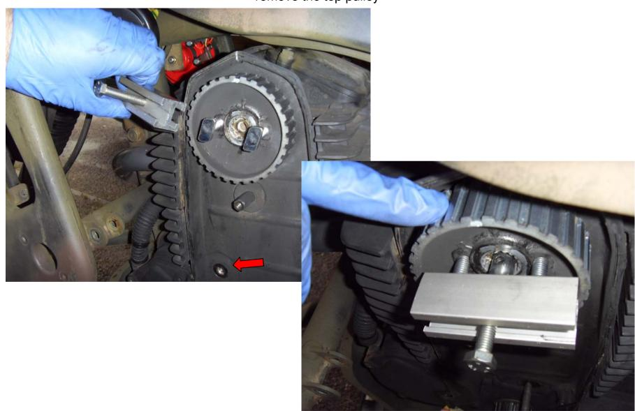
Using a 24mm socket remove the nut on the lower pulley I use a 75mm puller to remove the lower Pulley but there is a Rotax tool for the Job.
