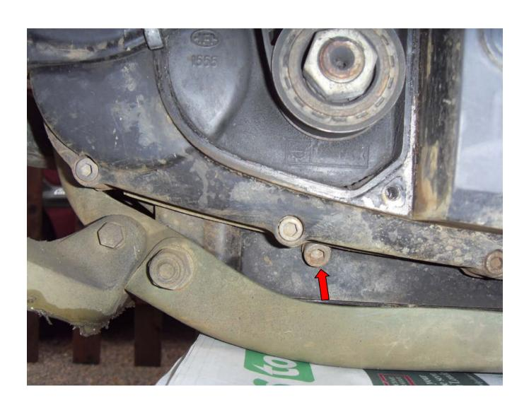
Screw in the crank Locking Bolt until finger tight then just nip it up this is all that is required to lock the crank.
