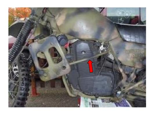
Using a 5mm Allen Key remove the Four Marked Cap Head Bolts
