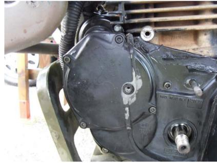
When replacing the lower Timing belt Pulley there are four Keyways place it back onto the shaft with the marked keyway up as in the Picture below I have used a slightly stronger alternative to the loctite 221 replace the nut and using a torque wrench tighten it up to 100NM
