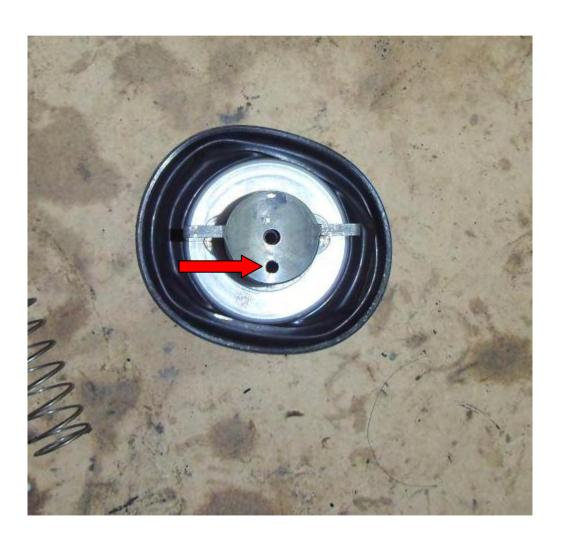
Below is the standard needle and the washers that I used the mod recommends 1.5mm raise but I used 2x 0.65 mm washers giving me a 1.3mm lift as this is all I could find all you have to do at this point is carefully slide the washers onto the needle
