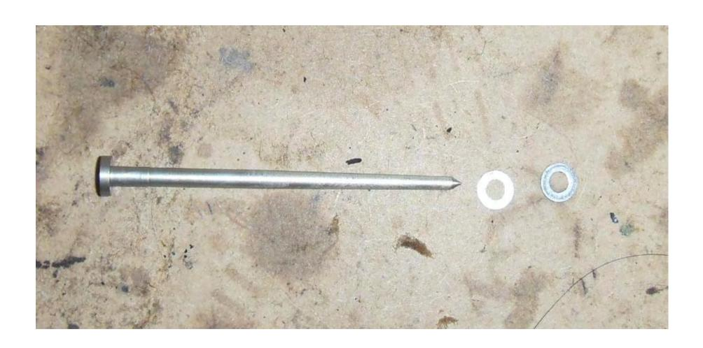
With the hole drilled and the washers placed on the needle the carb can be put back together I changed the 4 M4 screws on the top of the carb to cap head bolts as the screws used are like monkey metal and round off on the phillips section of them
