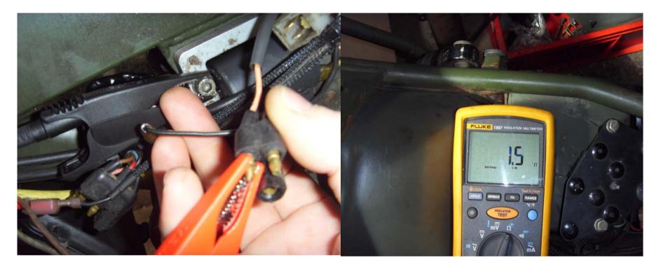
The Primary winding on the coil To test this I clipped the meter to a good Earth point and to the Pink cable as shown in the picture above This connector is on the Coil side not the amplifiers side
