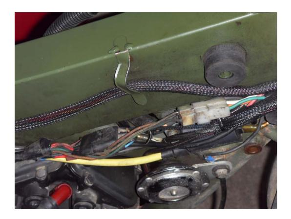
Once you have removed the seat and petrol tank using the 13mm Spanner it will give you access to the Connections you will need to unplug to test the resistances
