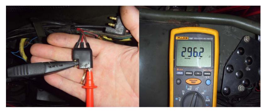
The Low Speed Charging coil To test this put a meter across the Brown and Black cables as shown in the picture above This connector is on the engine side not the amplifiers side
