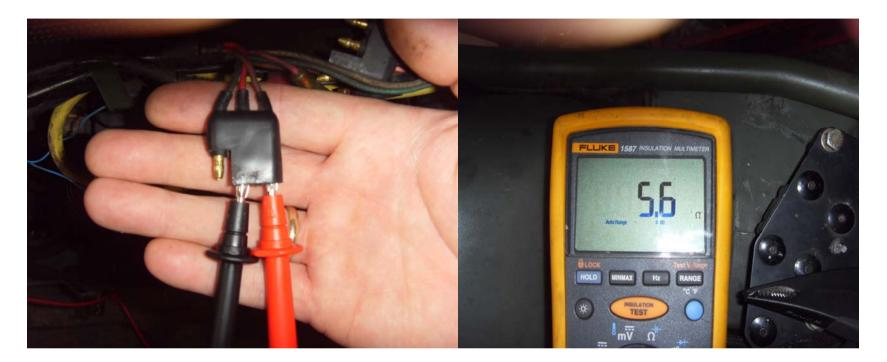
The High Speed Charging coil To test this put a meter across the Brown and Red cables as shown in the picture above This connector is on the engine side not the amplifiers side
