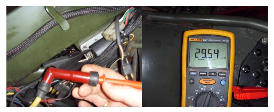
The Secondary winding on the coil
