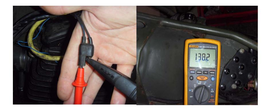
The Low Speed Trigger coil To test this put a meter across the Blue and Black cables as shown in the picture above This connector is on the engine side not the amplifiers side
