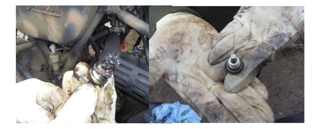
The Blue arrow is pointing to the Neutral light so you will need to move this out of the way The three red arrows point to the cap heads that you will need to remove to gain access to the oil filter Using a 5mm Allen key to undo the cap heads But do not remove them at this point
