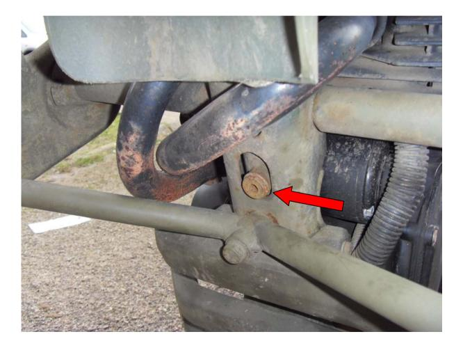
Once the oil has drained use some of the new oil to flush the bottom of the frame out
