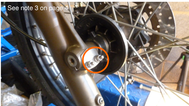
13. Tighten Spindle clamp Nuts (Pinch Bolts) to 12 Nm.
