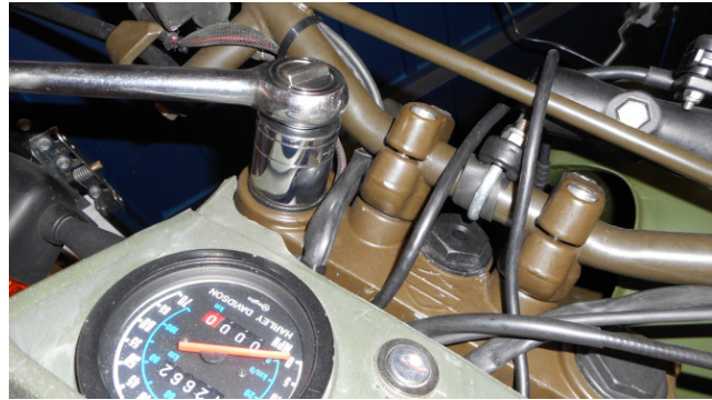
10. Replace both the fork cap assembly at the top of the forks.
