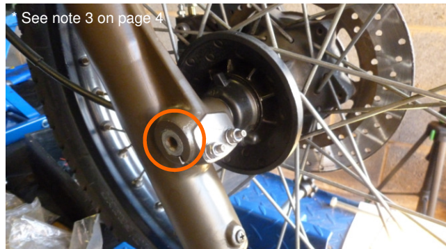
12. Insert wheel, spacer (left side) and front wheel Spindle. tighten to 68 Nm
