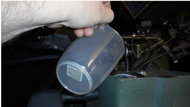
9. Fill forks with 475ml each of 15W Fork Oil (Note 500ml if fork has been rebuilt)
