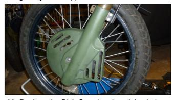
28. Replace the Disk Guard and retaining bolt
