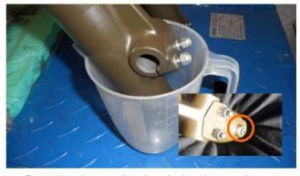
6. Put a bucket under the drain plug and unscrew and remove.
