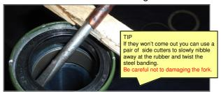
Under the seal there is a large steel washer (52) and the upper bushing (spacer 53) Which are left in position.
