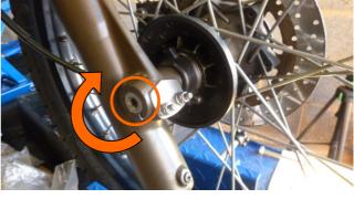
24. Insert wheel, spacer (left side) and front wheel Spindle.
