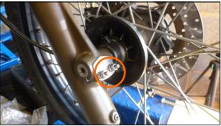
25. Tighten Spindle clamp Nuts (Pinch Bolts) to 12 Nm.
