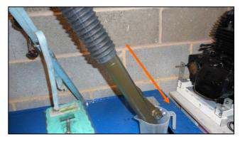
12. slide the lower fork down and out until it clears the fork riser.
