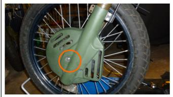
1. Remove the Disk Guard bolt (10mm spanner) and remove the plastic guard from the bike
