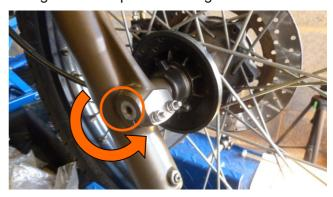
4. Remove the Front wheel spindle (axle) with an 8mm Allen key and remove the wheel.
