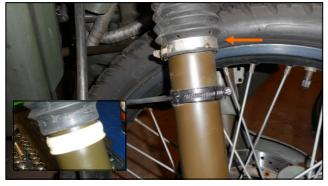
27. Replace the gaiter jubilee clips on both forks over the rubber gaiters and plastic retainers.
