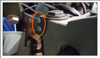
23. Tighten the Yolk Pinch bolts. If they were loosened to remove the cap
