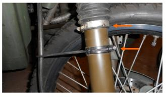
2. Remove the gaiter jubilee clips on both fork legs and the speedo cable guide
