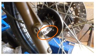
3. Loosen the Spindle clamp Nuts (Pinch Bolts) with a 10mm spanner
