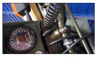
19. Insert the spring and pre loader If fitted.
