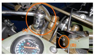
7. (A) Remove the fork cap assembly at the top of the fork (30mm Socket) and pull out the fork spring.
