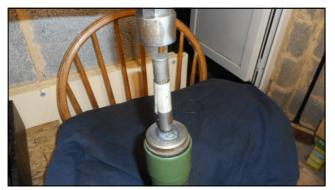
15. Place the seal in to the top of the fork with the flat part of the seal facing upwards.
