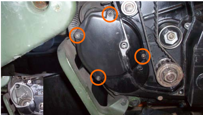
3. Remove the 4 bolts holding on the starter gear cover and remove the Cog & 2 washers.
