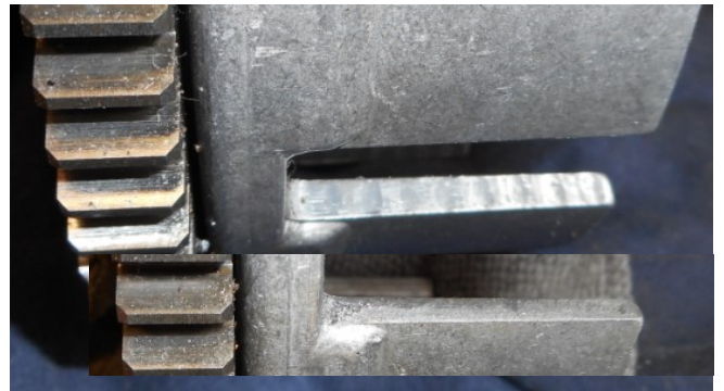
19. Check the Basket Spline's for Grooving and file down equally if required.
