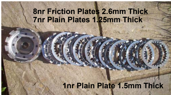
18. Remove the Friction and steel Plates and keep them in order as one of the plain rings is a different thickness. Re assemble with the new Friction plates and plain rings as required.
