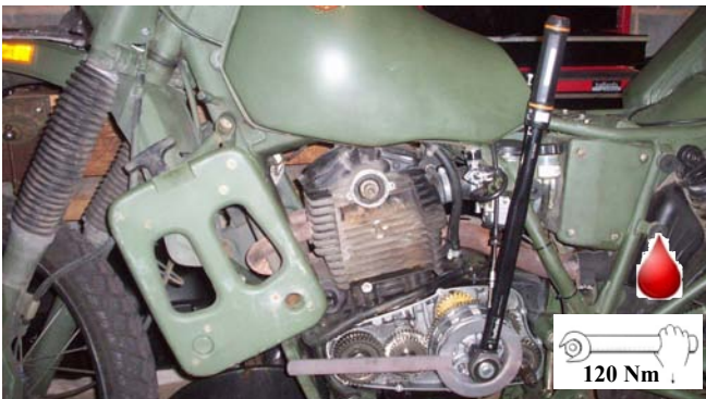
20. Replace the Basket and plates on the bike, then put the Clutch Hub, lock washer and the bolt on with " Strong thread lock " and torque up to 120 Nm .
