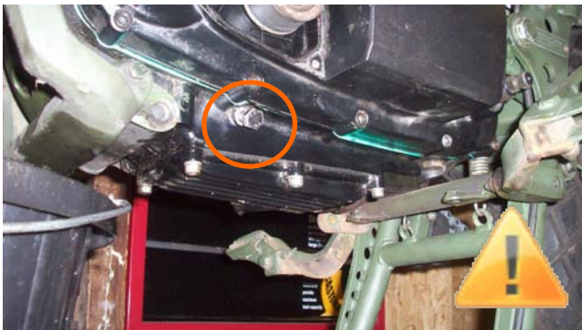
36. Remove the Fly Wheel Locking Bolt and replace with the original bolt & Copper Washer.
