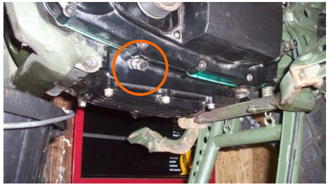
4. Remove the bolt circled above using a 6mm Allen Key . Locate the V in the fly wheel through the hole using a torch and screw in the crank locking bolt (the crank locking bolt is a M8 bolt with the end of the thread tapered.)
