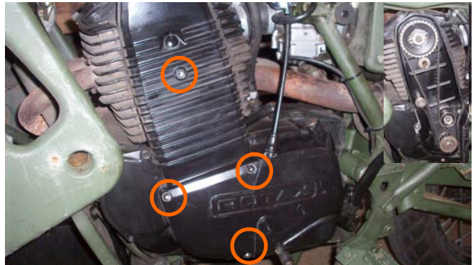
2. Remove the 4 timing cover bolts with a 5mm Allen Key. ( Note: Screws are Different Lengths)
