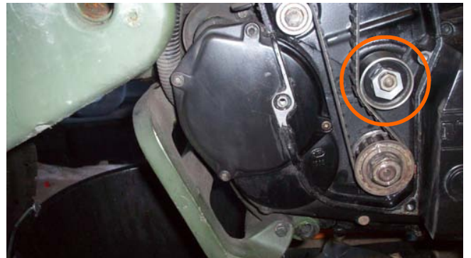
33. Refit the top Pulley and Spacers. Ensure the Two marks line up.
