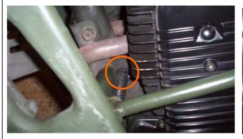
17. Remove the Primary Oil Filter clean and replace. This is very difficult to replace so I don't do this often. Remove necessary parts of the bike and replace as required.
