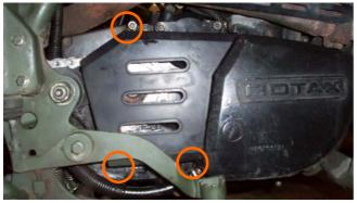
13. Re Fit the Plastic Chain / Sprocket Guard.
