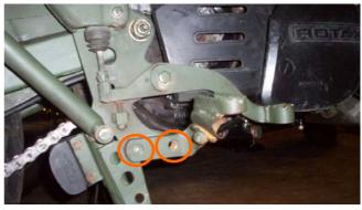
14. Refit the Foot Rest and tighten the 2 bolts to 24 - 27 Nm. 24-27 Nm.
