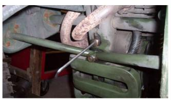
16. Replace the Drain Plug & Copper Compression Washer. Torque 20 Nm.
