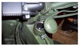
22. Replace the Filler Cap and check for any oil leaks on the parts and plugs removed and where the oil hoses connect to the engine / frame are tight fitting.
