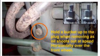
5. Remove the Oil Drain Plug with a 6mm Allen Key and drain out the oil. Run some fresh oil through to clean out the bottom of the frame. Clean the magnet plug of metal fillings. (Note: You can tuck a rag in below the plug to catch the oil from dripping down into the sump plate.)
