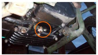
6. Remove the Sump drain plug and drain out the oil into the bucket.
