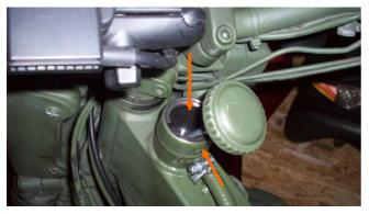
21. While running the bike ensure the oil is circulating by looking in the oil filler hole ensuring oil is returning through the return pipe.
