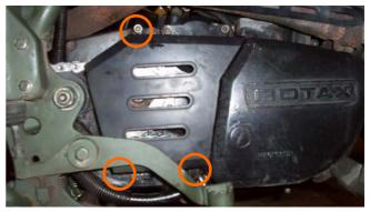
4. Remove the Chain & Sprocket Guard with a 5mm Allen Key.
