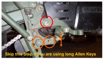
3. Take the right bolt out and loosen the left bolt to drop the Right Foot Rest. The Brake Pedal will need removing if you use short Allen keys.
