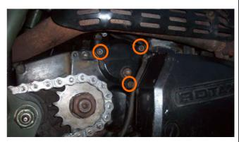
12. Replace the cover seal and Refit  $\operatorname{Sec}_{8 \mathrm{Nm}}$
