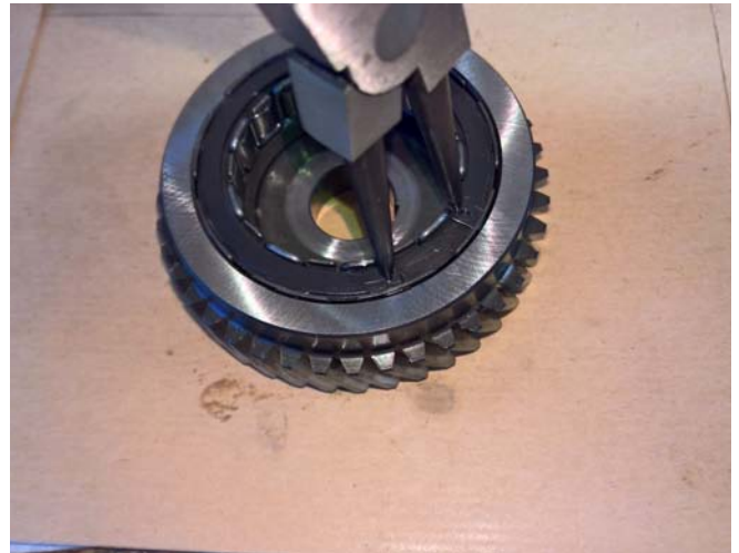
17. Using a pair of circlip pliers squeeze in the retaining circlip and pull the sprag out.
