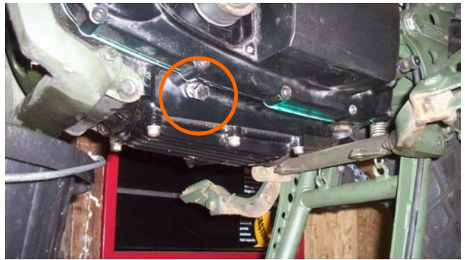
4. Remove the bolt circled above using a 6mm Allen Key. Locate the V in the fly wheel through the hole using a torch and screw in the crank locking bolt (the crank locking bolt is a M8 bolt with the end of the thread tapered.)
