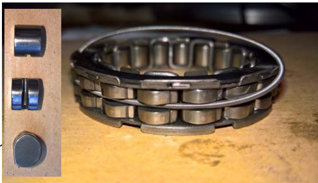
18. Replace the whole sprag unit, lobes or spring as required.
