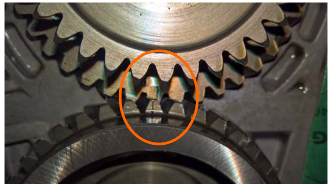
19. Reinstall the gear and align the marks if it was removed.
