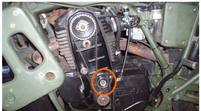
6. Remove the Timing Belt Tension bearing.
