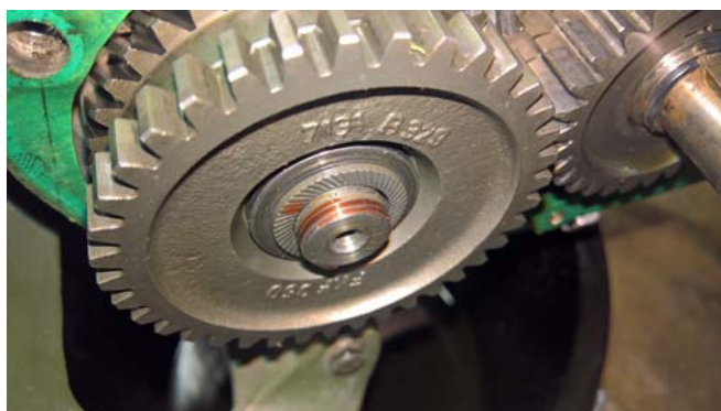
22. Reinstall the collar, bearing, cog, washer, lock ring & apply thread lock.
