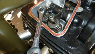
10. If the gap is not correct loosen the nut with a 11mm spanner.
