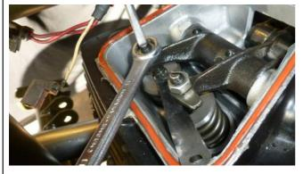
11. Using a screwdriver turn the adjuster until the feeler gauge fits in snugly and tighten the nut. (Then a final check on the gap)
