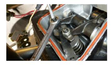
This is intended as a walk through & Guide only to the Valve Clearance on a MT350 / Rotax 348 engine
