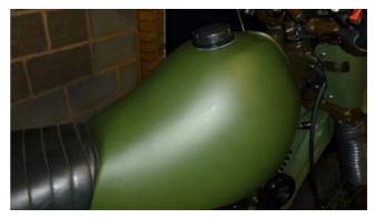
16. Replace the Fuel Tank & Fuel Hose Switch on the fuel (Check for any Leaks) Replace the Seat. Replace the Side Panel.
