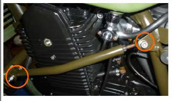
3. Remove the Support Strut
