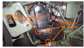
4. Remove the Timing Belt Cover (Not essential but makes it easier to turn the engine)
