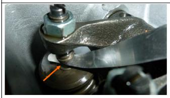
9. Using a 0.05mm Feeler Gauge check the gap.
