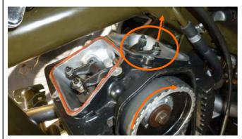
13. Turn the engine until the back rocker is in the up most position.(Inlet valves are in the fully closed position.)
