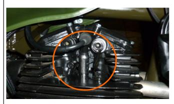
5. Remove the HT Lead and Spark plug. (Not essential but makes it easier to turn the engine)
