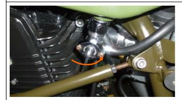
1. Switch off Fuel Tap, put the bike into Neutral and remove the Side panel.
