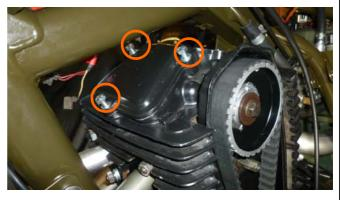
6. Remove the 3 Bolts on each of the two Valve Covers
