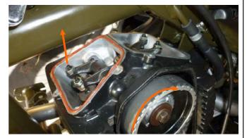
8. Turn the engine until the front rocker is in the up most position. (Exhaust valves are in the fully closed position.)
